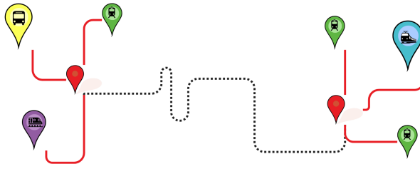
Figure 5: Link creation between the origin-destination pair and the closest stations to them
