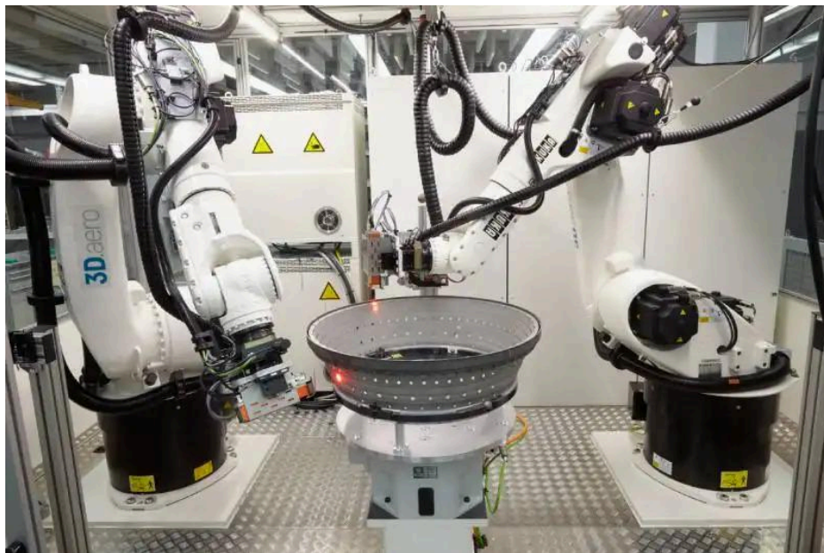
Figure 19. 3D.Aero's AutoInspect aerospace visual inspection system [93]
