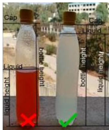
Figure 48. How Liquid class is used to classify emptiness of a bottle
