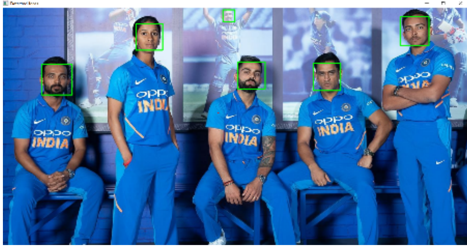
Figure 1.8: Result of Output image using Haar cascade [Geeb].
